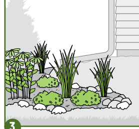
3 Install a rain garden to collect stormwater (at least 5 m from the foundation).
