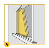
Install windows and doors with low Solar Heat Gain Coefficients, that let less heat in.
